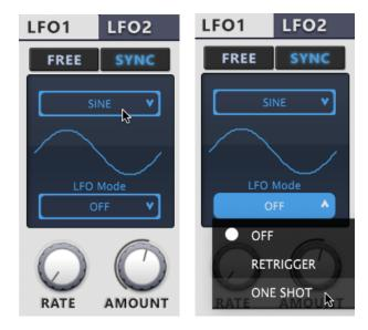
Ascension features 2 LFO's (low frequency oscillators), each with a choice of 5 waveforms, including a custom option, allowing you to draw your own LFO waveforms including smooth vector curves.
