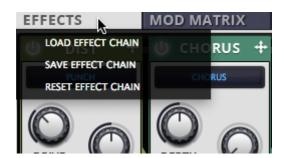
Right click the EFFECTS tab to load or save an FX chain, or reset the chain's configuration.
