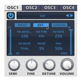
Lo / Hi: Filter out unwanted frequencies from each oscillator using high shelf and low shelf filters.
