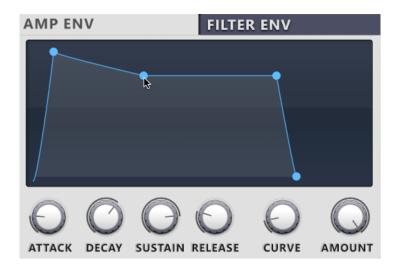
Ascension features a standard ADSR amplitude envelope. You can click each point to manipulate Ascension's envelopes with your mouse.
